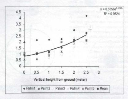
Fig. 5: Variation of PCA reading (LAI) with different height from ground to the lowest frond
