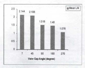
Fig. 8: PCA LAI variation with different view cap angle
